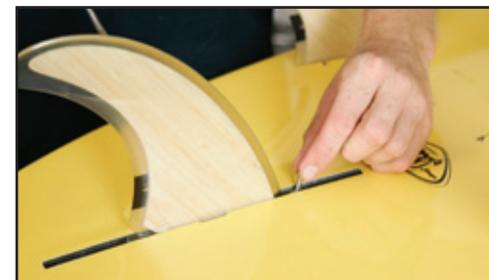
7) Insert the screw into the fin tab.
