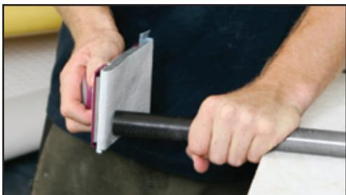
5) Remove the masking tape. Using the sanding block, sand the end of the shaft flat and smooth out the edge.
