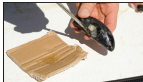
2) Coat the inside of the handle with the epoxy.
