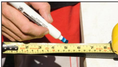
2) Using a fine tip permanent marker, mark a line on the shaft where you will make the cut.
