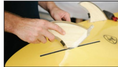
3) Holding the fin at an angle, insert the metal pin into the fin box opening.
