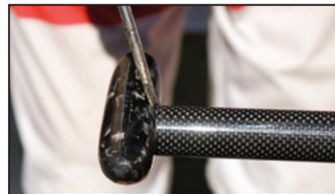
5) Once the handle has dried, drip a bead of epoxy around handle connection to prevent leakage.
