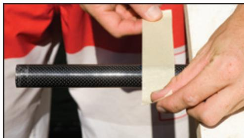
3) Wrap a strip of masking tape around the shaft where you put your mark to prevent splintering while cutting.
