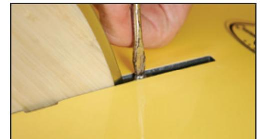
8) Using the screwdriver, tighten the screw into the underlying metal plate.
