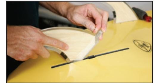
4) Keeping the fin at an angle, slide the fin into position.
